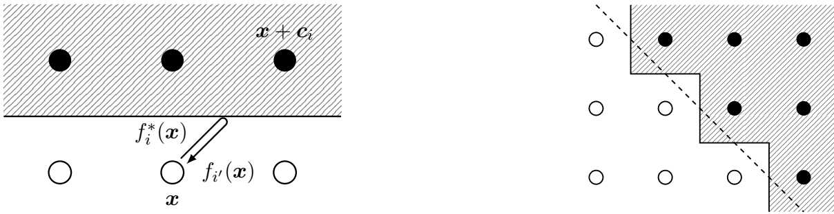
Figure 1: Bounce-back (left) is often applied for non-aligned walls. In this case, the boundary is approximated by a staircase (right).
